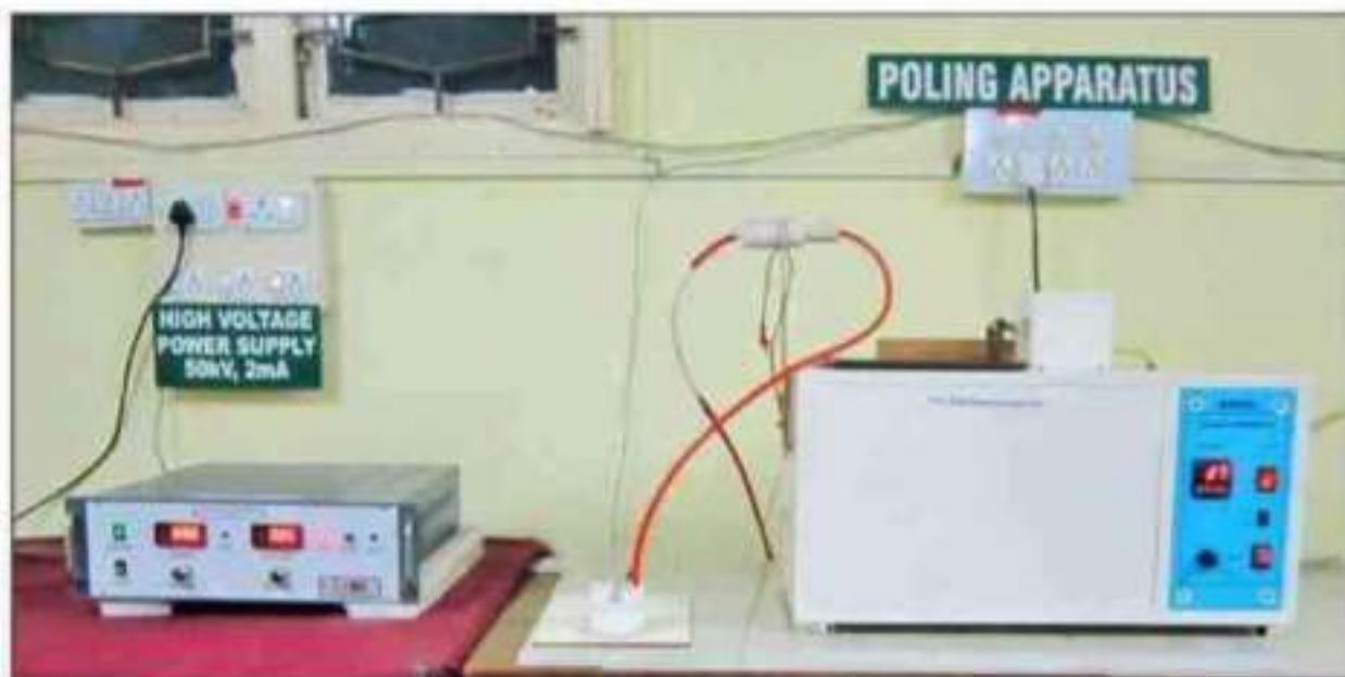
Poling Apparatus with High Voltage Power Supply
