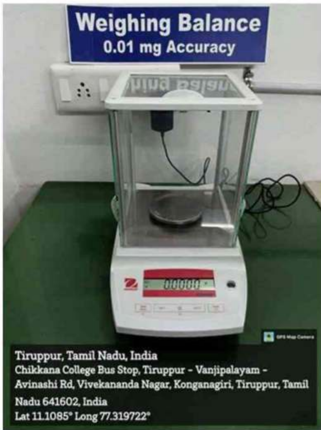
Weighing Balance 0.01 mg Accuracy
