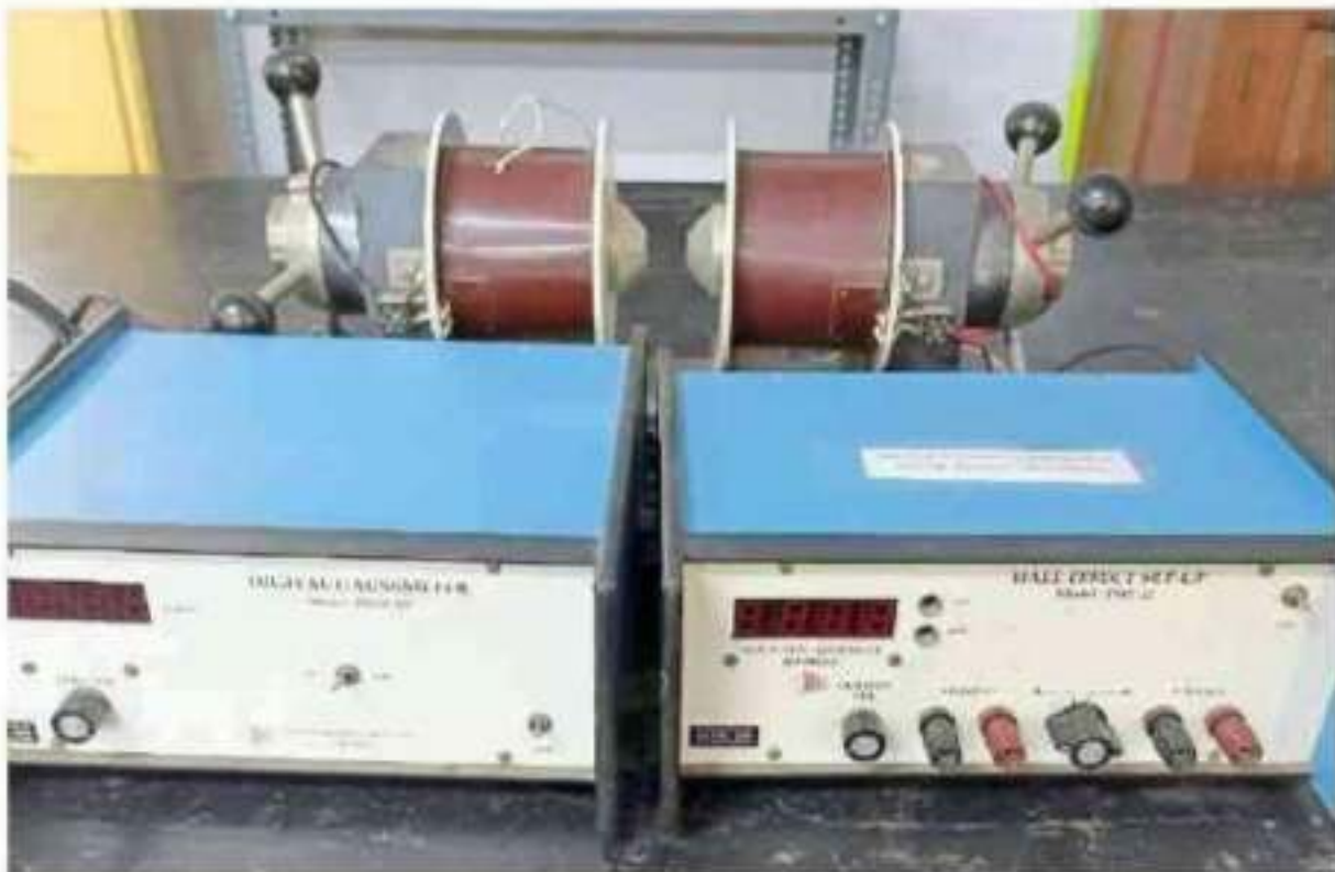
Hall Effect - Experimental Set-up
